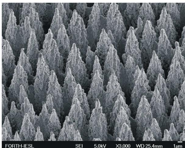
**Fig. 1** An example of a specially prepared and processed surface: ZnO thin films deposited with Pulsed Laser Deposition on a Si substrate whose surface has been treated with femtosecond lasers so as to form micro-cones.
