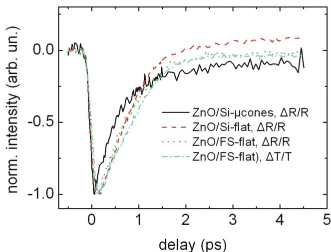
**Fig. 2** Ultrafast pump-probe measurements of ZnO thin films on flat and on micro-conical Si substrates. The dynamics in the micro-conical structures is faster due to the introduction of defects by the conical shape and the decorative protrusions [1].
